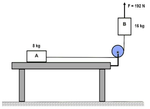
The kinetic frictional force acting on block **A** is 23,52 N. Ignore the effects of air friction.
