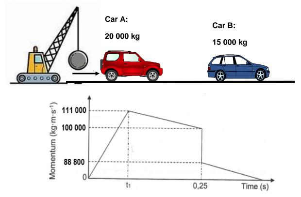
The momentum versus time sketch graph is drawn, as shown above, for car **A**. From the moment it is struck by the wrecking ball (t = 0 s), as it leaves the wrecking ball ( $t = t_1$ ) and as it collides with car **B** (t = 0,25 s).
