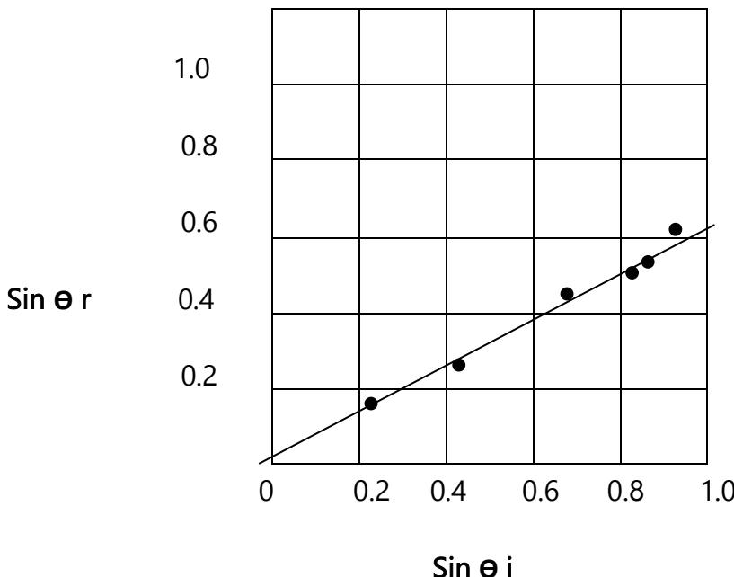
Slope of graph/Helling van grafiek =  $n = \frac{\Delta y}{\Delta x} = \frac{\Delta \sin r}{\Delta \sin i}$  OR  $n = \frac{\Delta \sin r}{\Delta \sin i} \checkmark$
